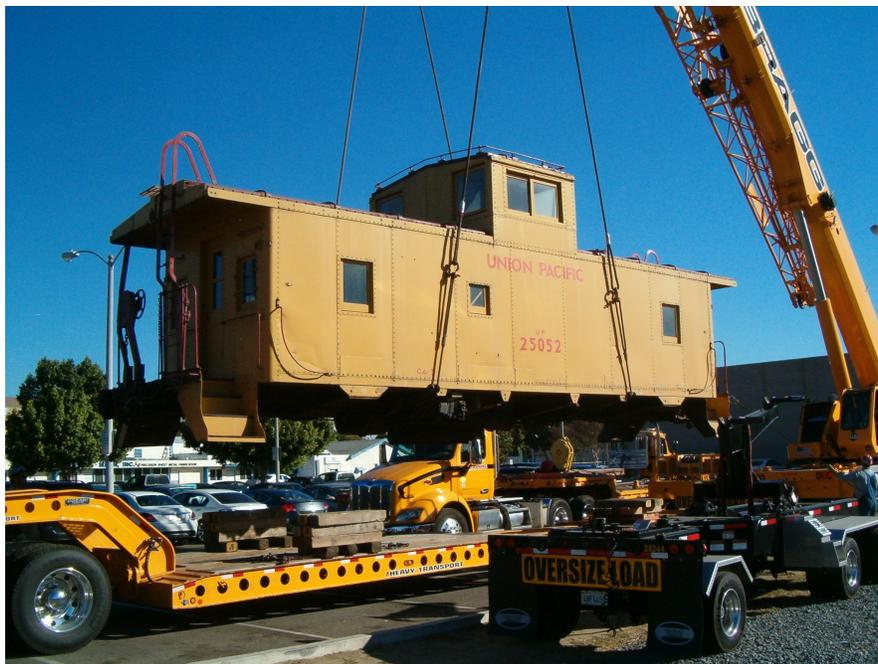
**Bragg Crane Company's "big hook" lifts caboose into position above its trucks at Fullerton Depot.**
