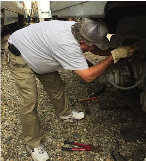
**Harold Benash removes locking wires for Bill Hatrick to inspect the wheels and bearings.**
