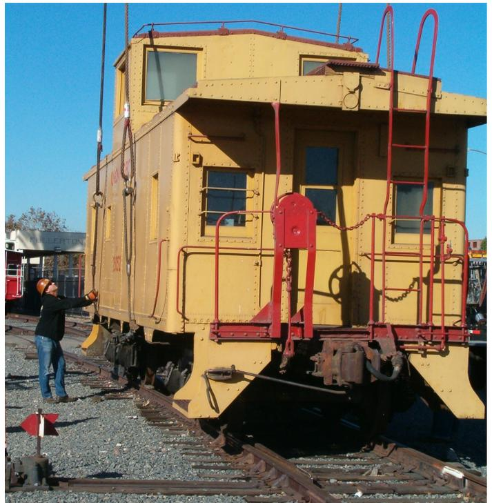
Bragg Crane "rigger" prepares to remove slings and complete the caboose lift into place on tracks.
